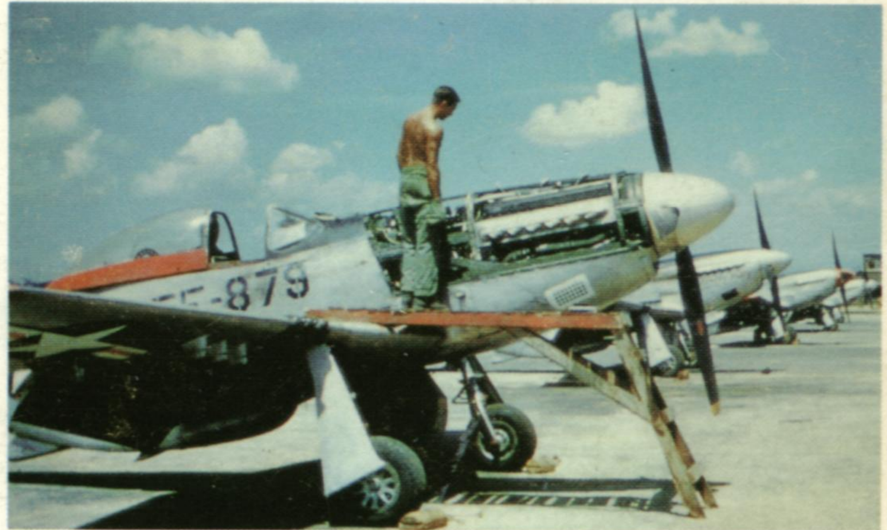
(Above) A 67th FBSq F-51D undergoing engine maintenance at Chinhae AB, Korea in the Fall of 1951. (Forbert)
