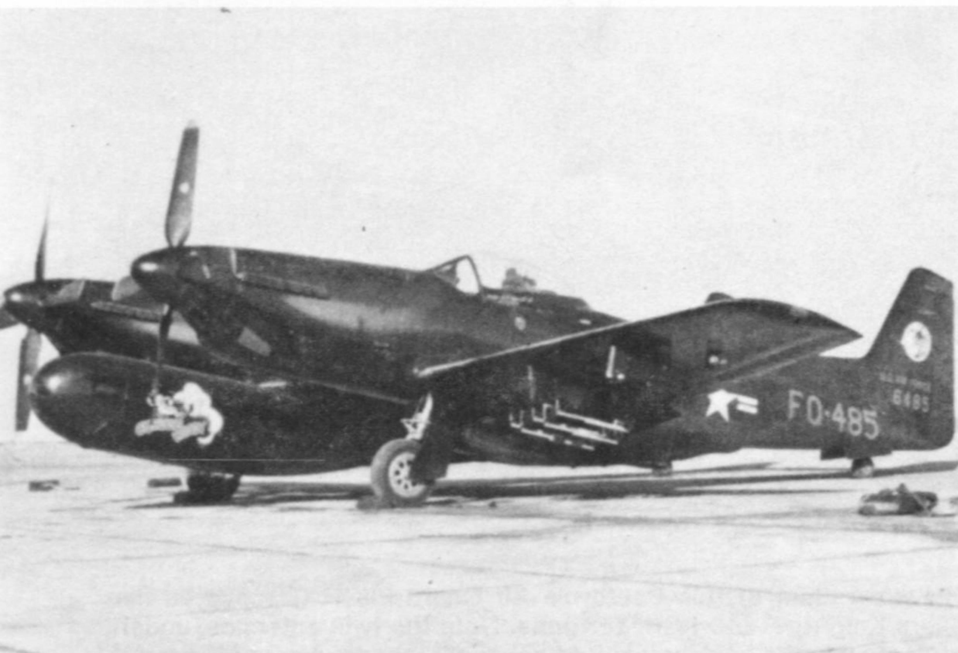
(Above) An F-82H from the 449th FISq at Elmendorf AFB, Alaska. The tail and outer wing panels are painted Arctic Red for higher visibility in case the aircraft was forced down in the snow covered coun-
