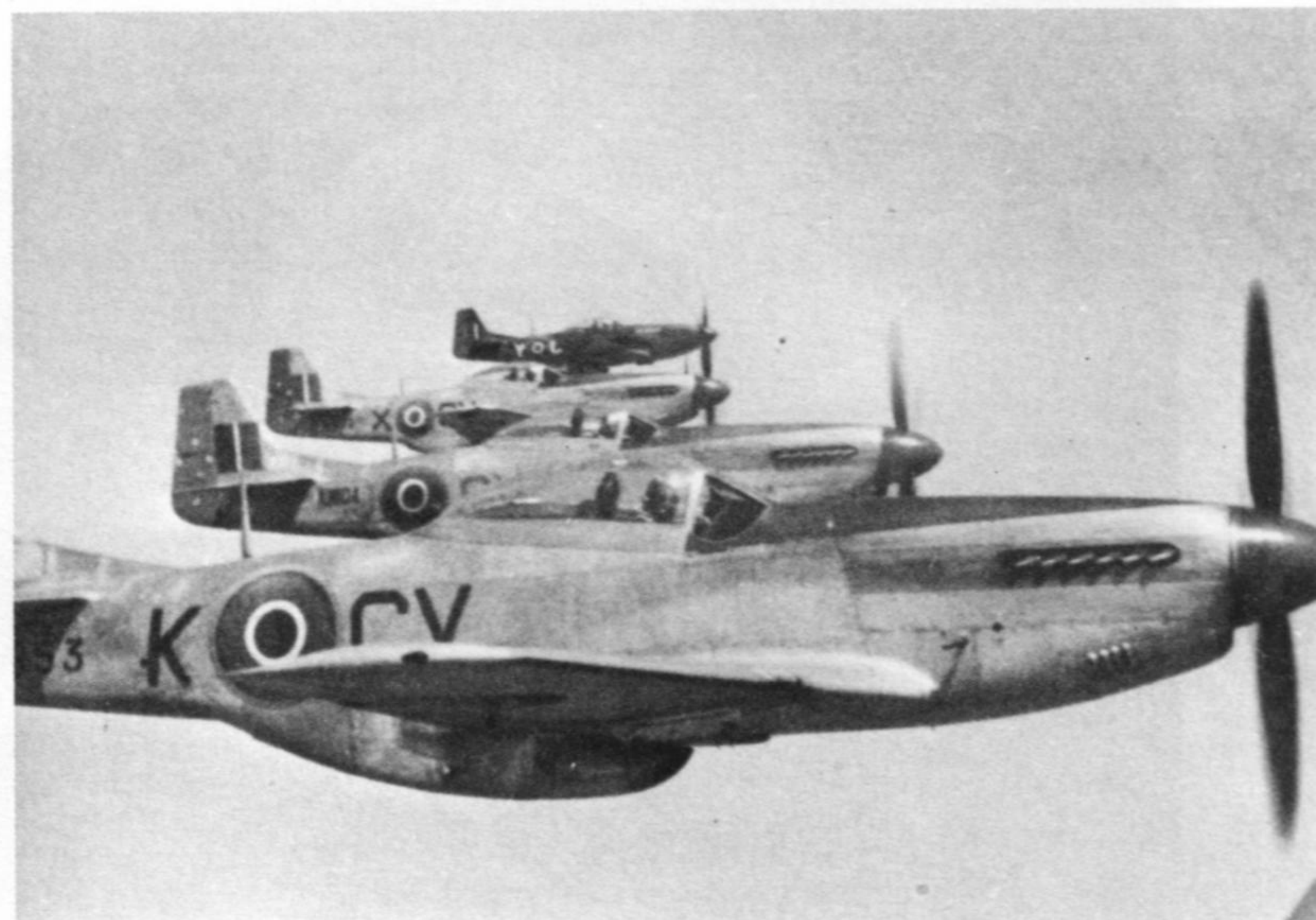
(Below) A flight of No. 3 Squadron, RAAF, Mustang IVs over Italy in 1945; three are in natural metal and the fourth is in the Dark Green/Ocean Grey camouflage. Note that Mustang IVs had louvered vent panels on the nose in place of the holes common on USAAF P-51s. (Smith via Ethell)
