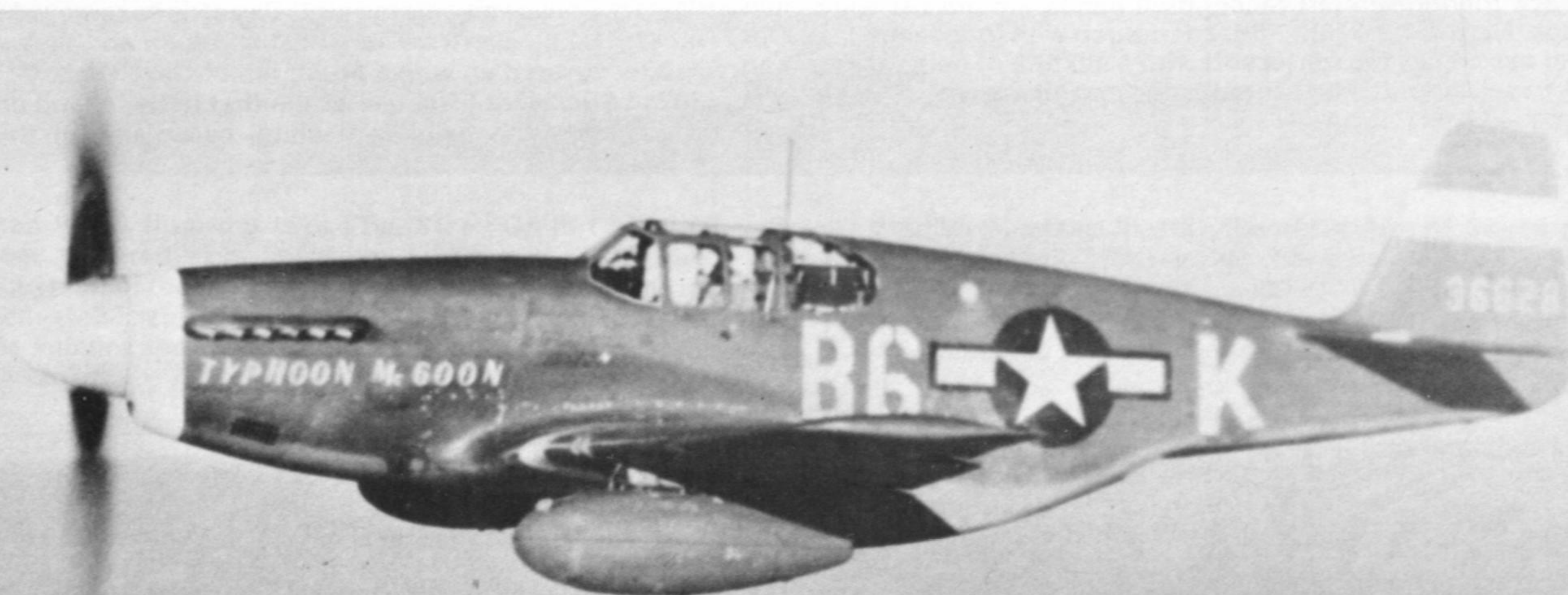
Typhoon McGoon from the 363rd FSq/357th FGp displaying the complete set of white friendly aircraft ID stripes on the nose, wings, horizontal and vertical tail. The code letters are in grey and the national insignia has been toned down with grey paint. (LePage)
